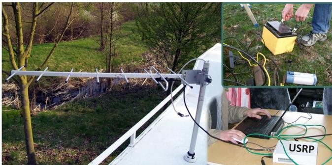
Figure 1. Mobile eavesdropping equipment. Left: Yagi-Uda antenna, connected to the data acquisition unit consisting of laptop and USRP in the measurement vehicle (right bottom); right top: voltage converter and car battery for the power supply in the wild.
