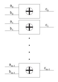
Figure 4.1: Addition in  $GF(2^m)$
