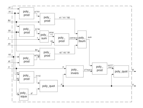
Figure 6.6: Block diagram of the calculation of A'(u) and B'(u) in parallel
