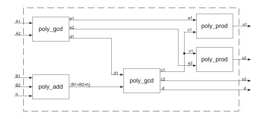
Figure 6.3: Block diagram of the calculation of *poly\_3gcd*
