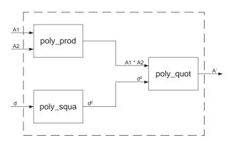
Figure 6.4: Block diagram of the calculation of A'(u)
