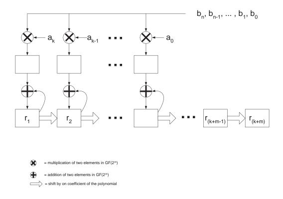
Figure 4.2: Block diagram of the polynomial multiplication
