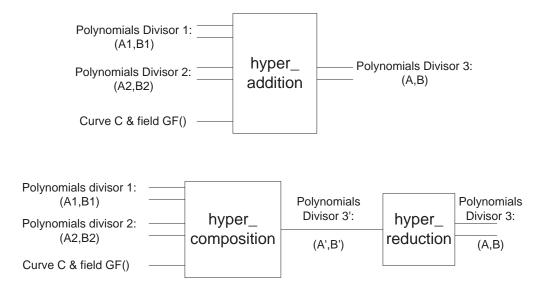
Figure 6.1: Block diagram for addition on Hyperelliptic Curves
