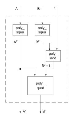
Figure 6.8: Block diagram of doubling
